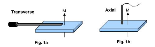
Next, ensure that you know the exact location of the Hall element within the probe. For example, when a certain gap is specified for testing, that is not the distance between the sample and probe end. It is the distance from the sample to the hall element located close the probe end. Gaussmeter equipment suppliers have data or drawings indicating the exact distance between the Hall element and the probe surface:
