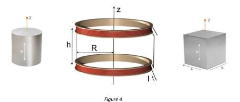
3. The Helmholtz Coil must be located for minimal outside magnetic interference. It is advisable to keep magnets at a proper distance from the coil and to avoid placing it on or near a metal surface. Even wearing a metal watch when testing can influence the measurement.
