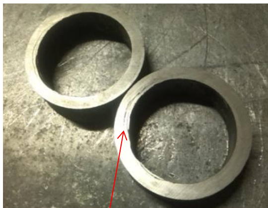
Crack during pressing
