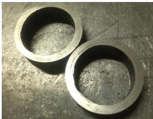
Crack during pressing
