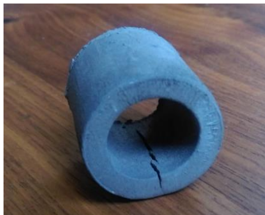
Crack after sintering
