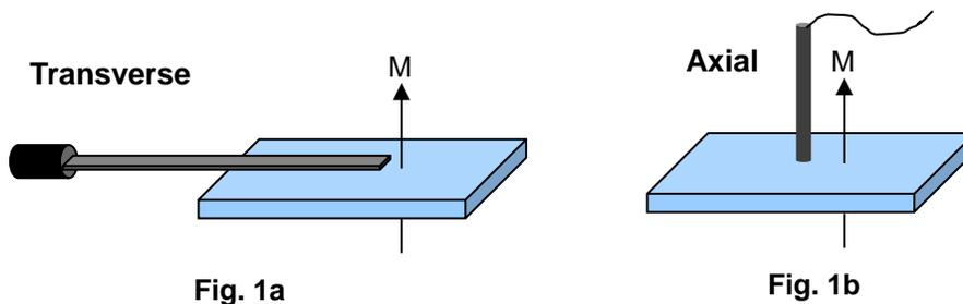
Next, ensure that you know the exact location of the Hall element within the probe. For example, when a certain gap is specified for testing, that is not the distance between the sample and probe end. It is the distance from the sample to the hall element located close the probe end. Gaussmeter equipment suppliers have data or drawings indicating the exact distance between the Hall element and the probe surface:
