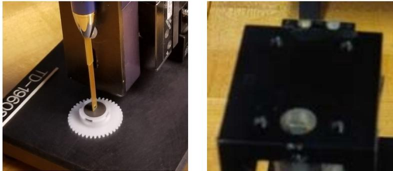
When measuring, please keep in mind that the probes are sensitive to any other magnetic devices nearby. You should keep the lot of samples several feet away from the location of your probe and only bring one magnet at a time to measure. Verify that there is no metal nearby or underneath the probe fixture as that will affect the accuracy of your test.
