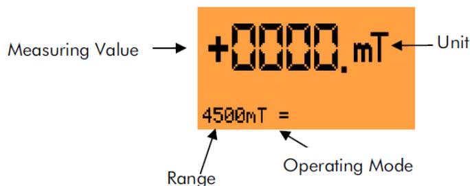
Before starting sample measurements, the probe and meter need to be “zeroed” or calibrated to a known magnetic reading. Suppliers of this equipment often include a Zero Gauss chamber or a calibration magnet sealed inside a closed circuit to protect its magnetic reading. When the probe is placed inside a Zero Gauss chamber, press the Null or Zero button on the Gaussmeter. After a few seconds, your unit will be ready for testing.
