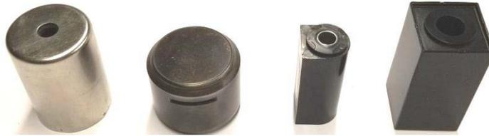
Once the equipment has been zeroed or calibrated, testing can begin by accurately placing the probe where you need the magnetic measurement. The sensing element measures only the lines of flux that are perpendicular to it, therefore it is important to note that any slight change in angle or location of the probe in relation to the magnet being tested will yield different results. For measuring large numbers of samples, simple fixtures can be made out of non-magnetic material.
